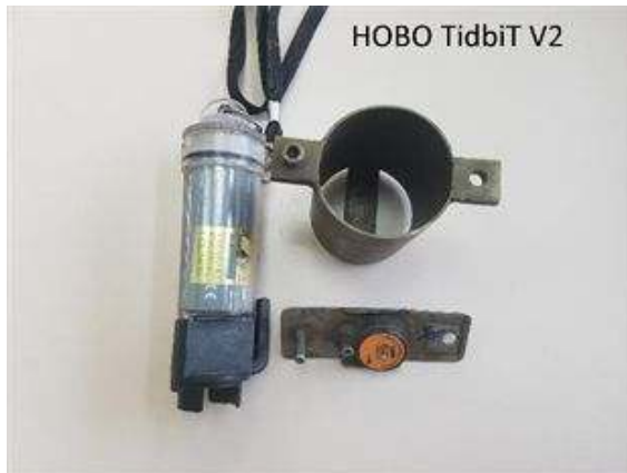
Photo 4 HOBO V2 water temperature logger introduced. ◦ More memory, ◦ more accurate, ◦ computer replaced with handheld reader. ◦ Disadvantage - data can't be checked or seen in field.
