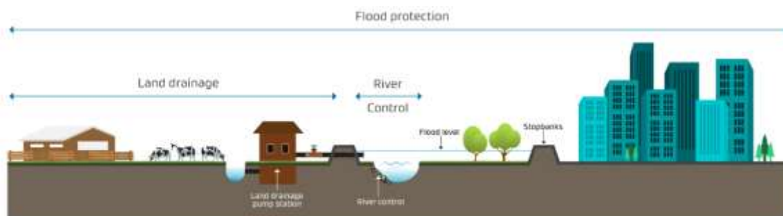
Figure one: Schematic of river management, flood protection, land drainage services (Source: Tonkin and Taylor, March 2018)
