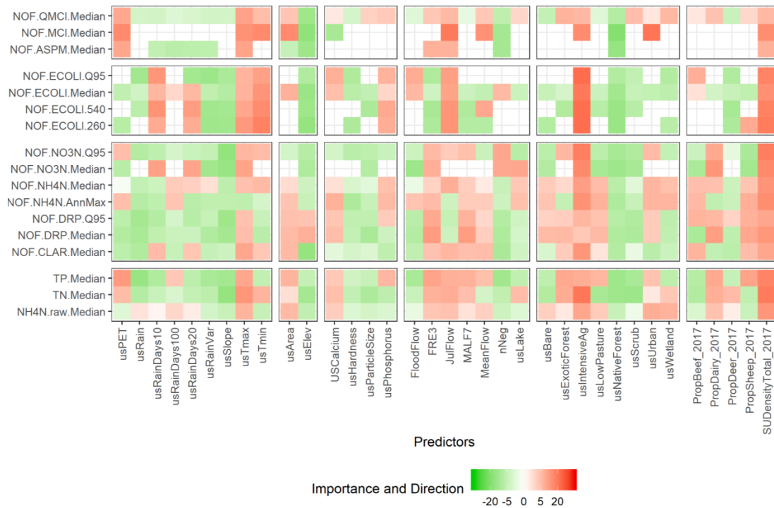
Figure 4: Relationships of predictors included in the ‘reduced’ random forest models with the water quality compliance statistics. Colours indicate the importance and direction of influence of each predictor on the modelled state statistics. Red indicates increasing predictor magnitudes are associated with increasing values of the state statistics, whereas green indicates increasing predictor magnitudes are associated with decreasing values. Blank cells indicate that the predictor was not included in the “reduced” random forest model.
