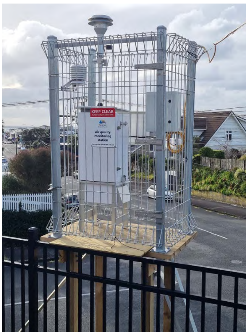
Figure 10 The new BAM1022 monitoring set-up at Central School. July 2022
