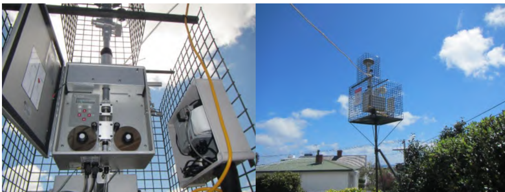
Figure 2: The original E-BAM monitoring system set-up and installation at Central School, New Plymouth. This equipment was upgraded in July 2022.
