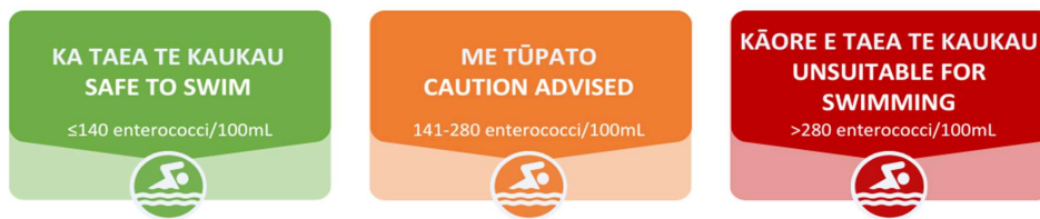
Figure 4: Guideline enterococci values for swimming and recreation at marine and coastal sites.
