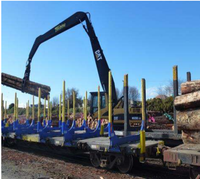
Figure 9: Loading logs at Palmerston North
