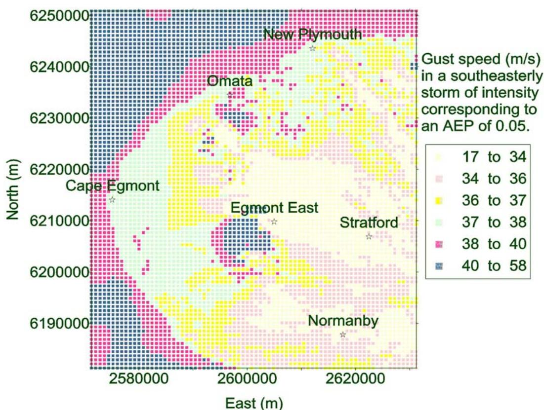
**Figure 2.** Maximum gust speed (m/s) at 10 m above ground determined by a numerical model run on a grid spacing of 800 m and extending to 7000 m above the ground. Mt Taranaki is in the lower central part of the grid. © NIWA
