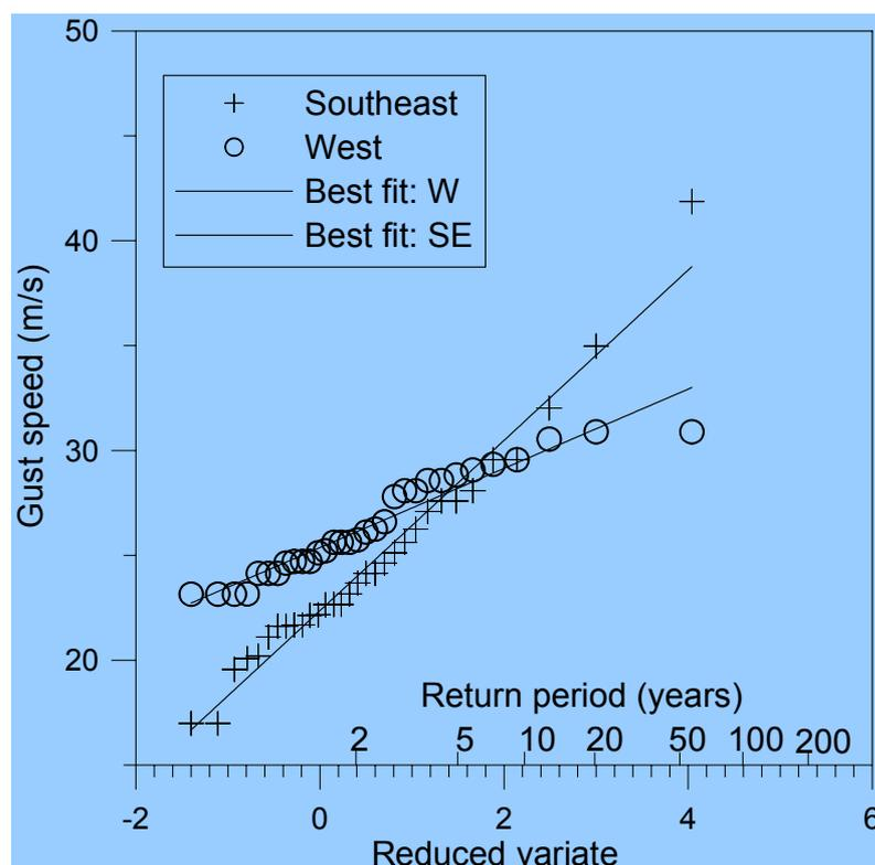
Figure 4. Gumbel plots of the annual maximum gust speeds at New Plymouth from the west and southeast directions. © NIWA
