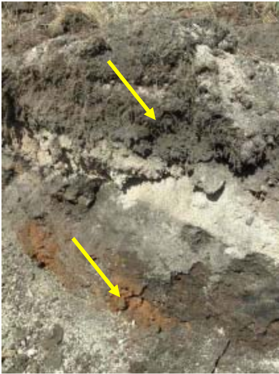
Pit 2 (829 & 830) 2637622-6159215 Layer of pumice 0.2-0.3m, then dark layer 0.3-0.5m (sampled) and friable red material (sampled at 1.5m).
