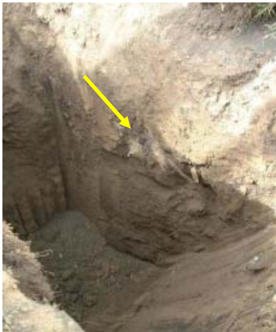
Pit 4 (822) 2637396-6159372 Natural ground at 1.5m, sampled dark material at 0.5m.
