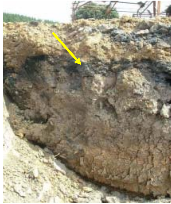
Pit 8 (826) 2637388-6159422 Sampled dark band at 0.2-0.3m, pit had been dug north of the northwest corner of the main reservoir.
