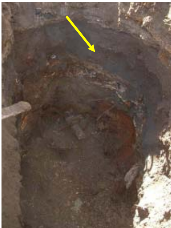
Pit 1 (828) 2637624-6159206 Fill to bottom of hole at 3m, sampled dark material at 1.5m.
