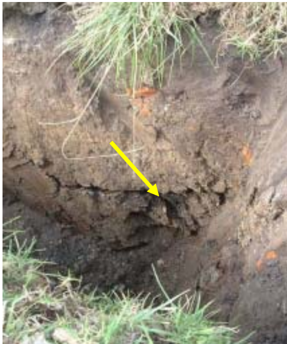
Pit 1 (821) 2637361-6159383 Natural ground at 2.5m, sampled dark material at 1.5m, noted rubble/debris.
