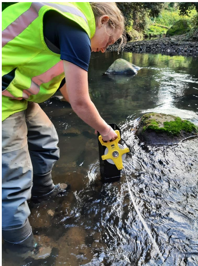
Photo 3 Monitoring of suspended fine sediment by black disc visual objectives.
