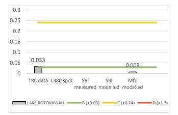
Figure 34: Measured and modelled data for ammonia (toxicity) (mg NH<sub>4</sub>N/L) at Lake Rotokawau (median)
