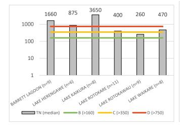
Figure 6: Median values for total nitrogen (mg/m<sup>3</sup>) at six Taranaki lakes up to July 2023
