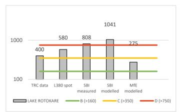
Figure 15: Measured and modelled data for total nitrogen ( $mg/m^3$ ) at Lake Rotokare
