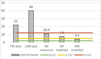
Figure 27: Measured and modelled data for chlorophyll-a (mg chl-a/m<sup>3</sup>) at Lake Rotokare
