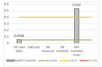
Figure 36: Measured and modelled data for ammonia (toxicity) (mg NH<sub>4</sub>N/L) at Barrett Lagoon (95<sup>th</sup> percentile
