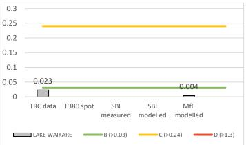
Figure 35: Measured and modelled data for ammonia (toxicity) (mg NH<sub>4</sub>N/L) at Lake Waikare (median)
