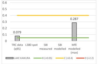
Figure 38: Measured and modelled data for ammonia (toxicity) (mg NH₄N/L) at Lake Kailkura (95<sup>th</sup> percentile)
