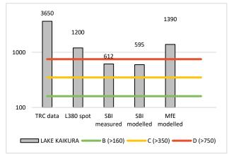
Figure 14: Measured and modelled data for total nitrogen (mg/m<sup>3</sup>) at Lake Kaikura
